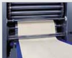
Reducing steps for a consistent, quality dough sheet (width and thickness)
