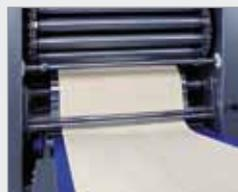
Reducing steps for a consistent, quality dough sheet (width and thickness)
