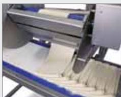
Laminating the dough-sheet (up to 512 layers) depending on the line concept
