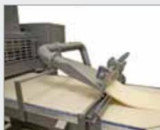
Fat-pump turns blocks of butter, margarine or zero-trans fats into a consistent sheet
