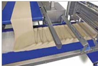
The belt with the dough sheet moves back and forth above the next conveying belt, this is an asymmetric lamination system. Suitable for soft dough and no restrictions regarding laminating width.
