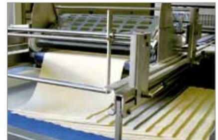
A guillotine cuts the dough sheet into regular rectangular sheets which are then stacked on top of each other. This flexible symmetric system lays even and uneven layers. Suitable for soft doughs and no restrictions regarding laminating width.
